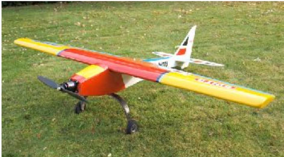
Micks electric Wot 4 which used to be powered by Saito 56 four stroke.
